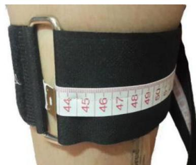
Figure 5 – Metal strap with ruler to measure the circumferences
