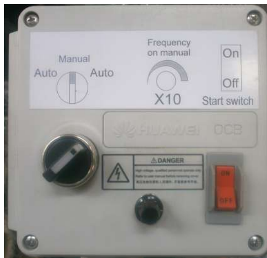
Figure 2 – Remote control of the feed rollers
