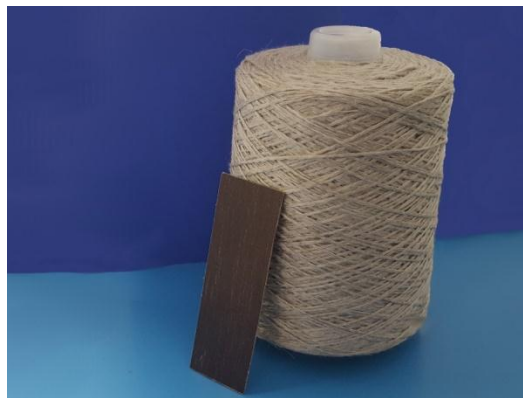
Figure 1 – Prepared linen roving and composite material formed using it
